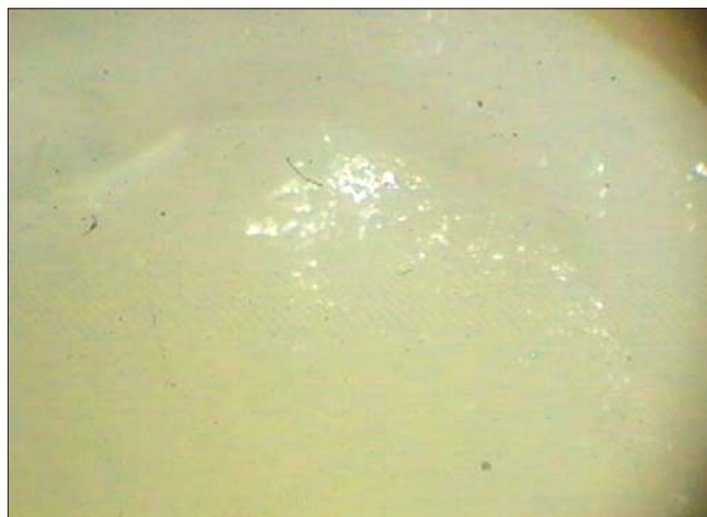
Figure 3: Combined (adhesive and cohesive) failure
