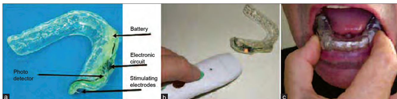
Figure 2: Second-generation removable device consists of three components: A miniaturized electronic stimulator that has a signal generator, power source and conducting circuitry; an intraoral removable appliance; and an infrared remote control. The miniaturized electronic stimulator is mounted in a removable intraoral appliance (a); which is under remote control that activates the stimulator (b); This device is applied into the mouth in a non-invasive manner (c)
