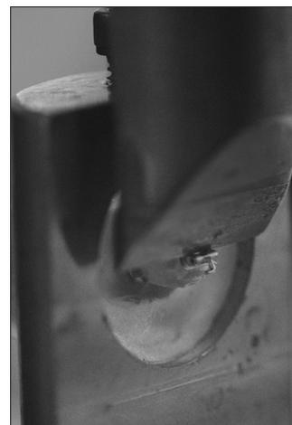
**Figure1:** Buccal tube and porcelain crown positioned for the debonding exercise
