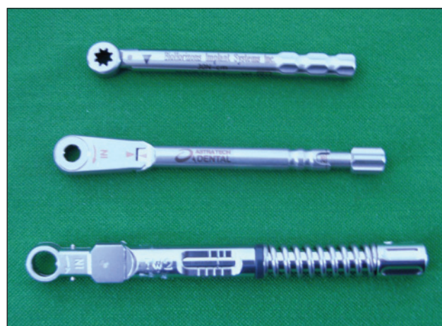
Figure 1: Friction-style mechanical torque limiting devices tested. X, Astra Tech — Y, BioHorizons — Z, Dr Idhe mechanical torque limiting devices
