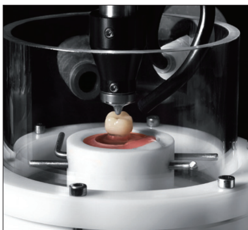
Figure 1: Load cycling was performed by chewing stimulator (SD Mekanotronik, Germany) equipped with an oral environmental chamber
