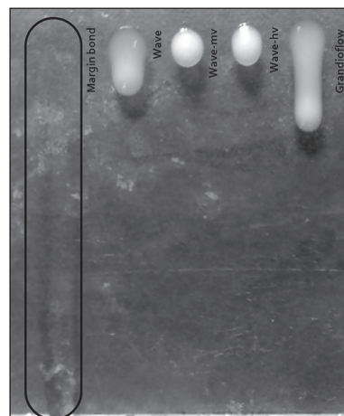
Figure 5: Flow of bonding agents which were used in this study at 90° angle for 5 min
