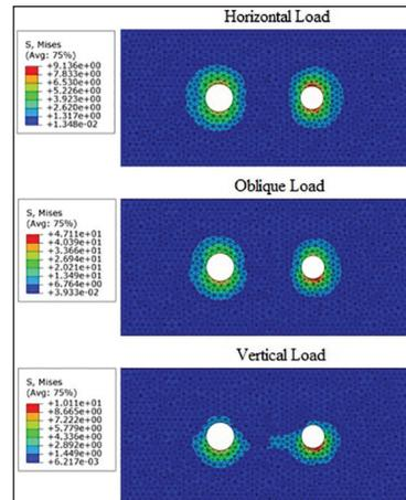
**Figure 3:** Von Mises stress values (MPa) and distribution patterns on the cortical bone when the different loads were applied
