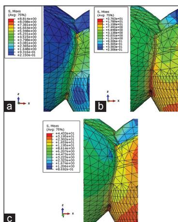
**Figure 7:** Stress distribution in connector regions (a) horizontal, (b) oblique, (c) vertical
