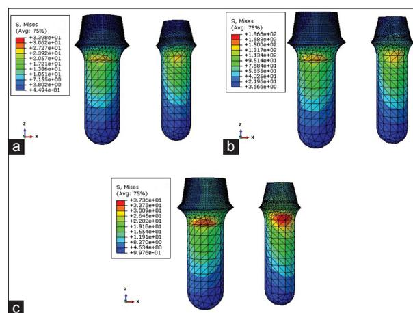
**Figure 8:** Stress distribution in implant and abutment regions (a) horizontal, (b) oblique, (c) vertical
