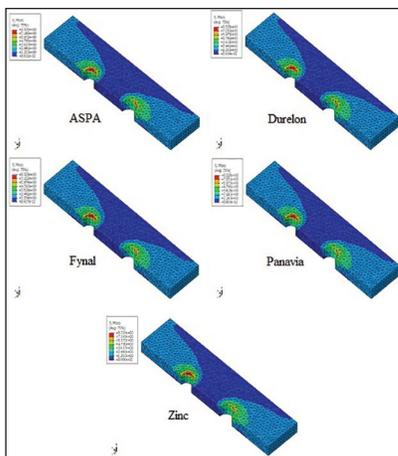
**Figure 4:** Comparison of applying different types of luting agent materials to cortical bone stress distribution (horizontal load)
