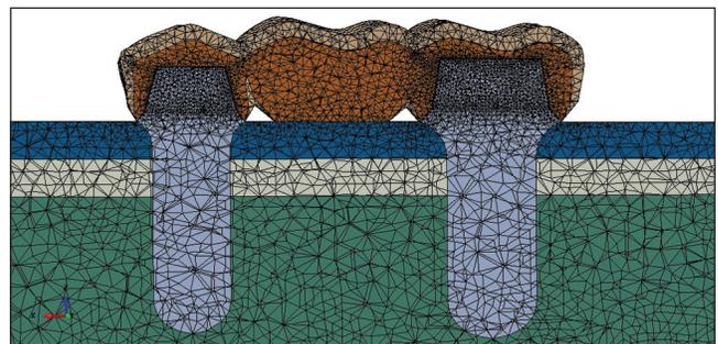
**Figure 1:** The geometric mesh of the modeled fixed dental prosthesis
