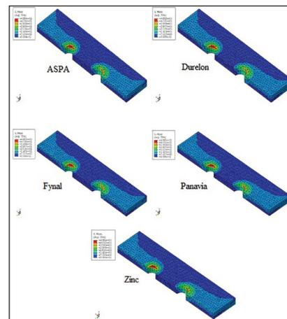
**Figure 5:** Comparison of applying different types of luting agent materials to cortical bone stress distribution (oblique load)
