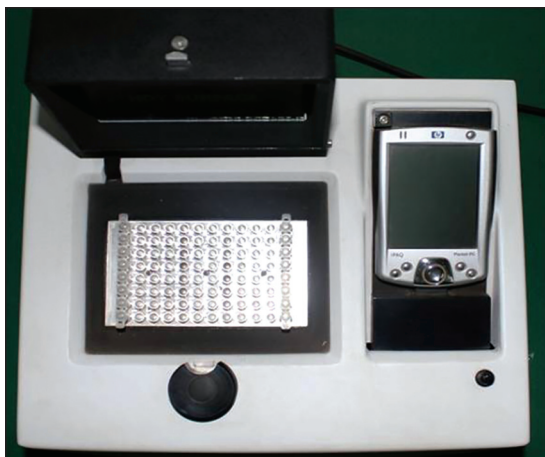
Figure 5: Conventional polymerase chain reaction thermal cycler
