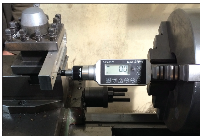
Figure 1: Torque testing setup (milling machine, torque tester, custom-made screw driver, mini-screw and polycarbonate plate).
