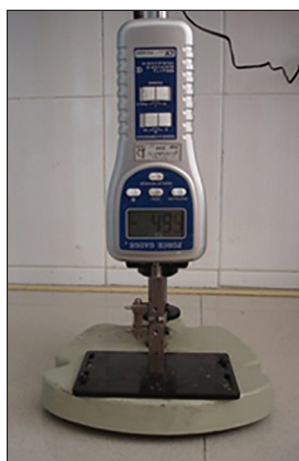
Figure 2: Force gauge coupling with jig. The distance between the posts remained constant while transferring to gauge.
