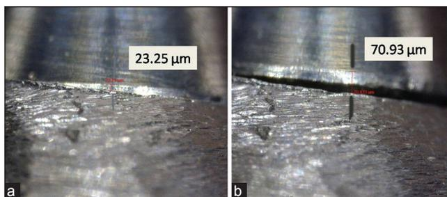
**Figure 2:** Vertical marginal discrepancy of the buccal side of one of the angulated abutment retainers following 20 (a) and 35 Ncm (b) torque tightening ( $\times 250$ ).
