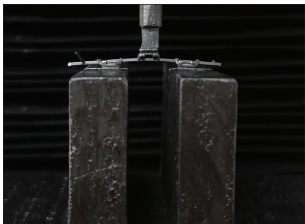
Figure 1: Universal testing machine set up while wire deflected 1.5 mm in anterior view.
