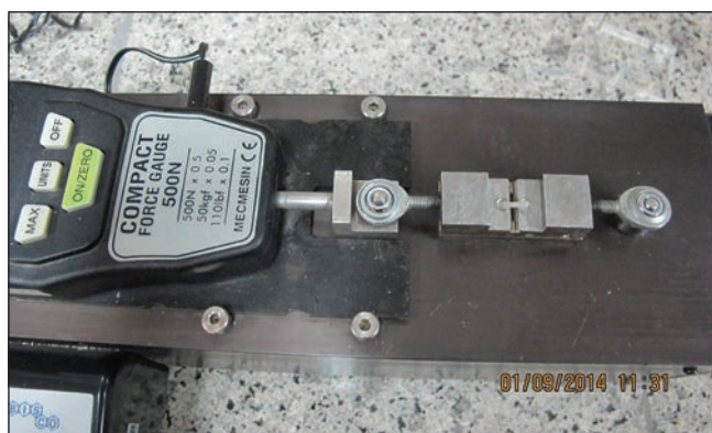
Figure 4: The tensile test machine.
