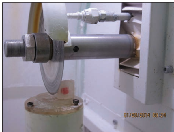
Figure 3: The composite specimen (red) merged in transparent acrylic resin.
