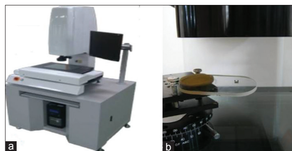
Figure 1: (a) Video measuring machine (automatic noncontact video measuring system, CAM series, ARCS Precision Technology Co., Taiwan). (b) Using special revolvers under the brackets for positioning them.
