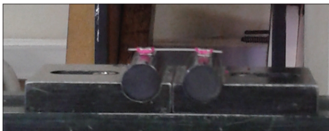
Figure 2: Close up view of the jig with two brass rods and brackets in place.
