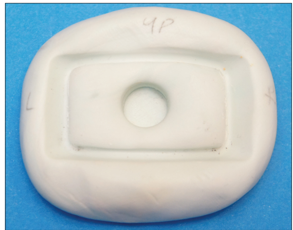
Figure 1: Representative the mold as a seat of the substrates and specimens for spectrophotometry.
