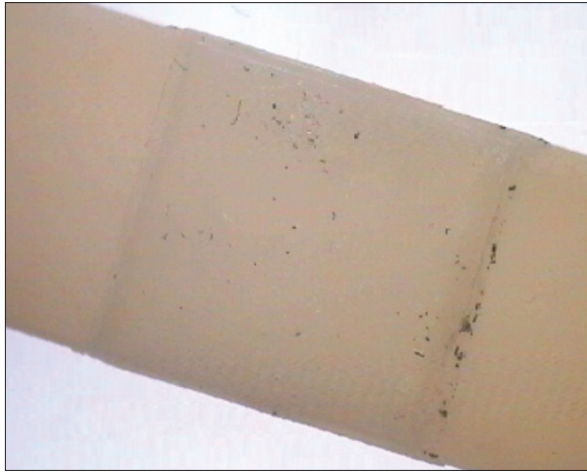
Figure 1: Cohesive failure occurred in 100% of the cases.
