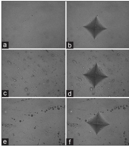
**Figure 2:** Photomicrographs of Admira Fusion before and after immersion in acidic drink for 1 and 7 days (x40). (a and b) Before immersion; (c and d) after immersion in acidic drink for 1 day, (e and f) after immersion in acidic drink for 7 days.
