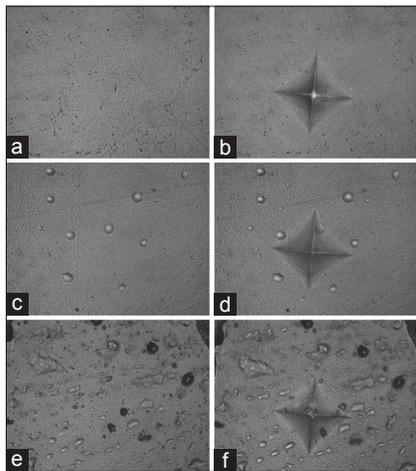
**Figure 3:** Photomicrographs of Ceram X Universal before and after immersion in acidic drink for 1 and 7 days (x40). (a and b) Before immersion; (c and d) after immersion in acidic drink for 1 day, (e and f) after immersion in acidic drink for 7 days.
