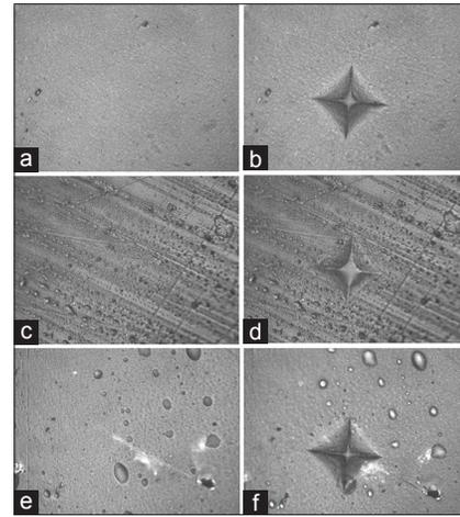
**Figure 4:** Photomicrographs of Filtek Supreme XTE before and after immersion in acidic drink for 1 and 7 days (x40). (a and b) Before immersion; (c and d) after immersion in acidic drink for 1 day, (e and f) after immersion in acidic drink for 7 days.
