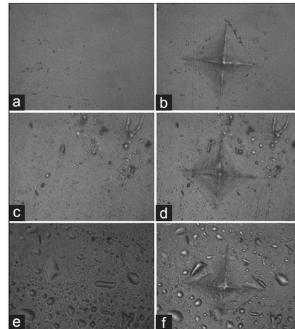
**Figure 5:** Photomicrographs of Gradia Direct before and after immersion in acidic drink for 1 and 7 days (x40). (a and b) Before immersion; (c and d) after immersion in acidic drink for 1 day, (e and f) after immersion in acidic drink for 7 days.
