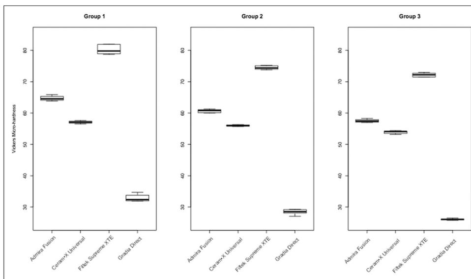
**Figure 1:** Box-plots for Vickers microhardness of material tested for each experimental group. Bold horizontal line represents median.
