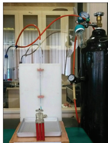
Figure 1: Fluid infiltration system.
