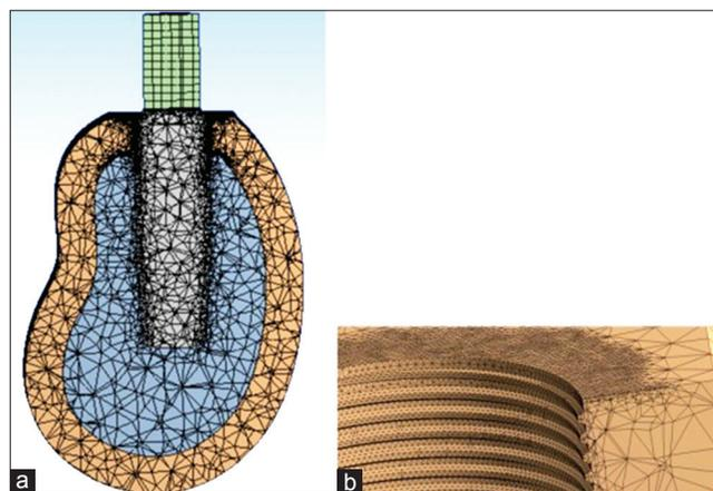
**Figure 2:** Cross-sectional view of the meshed model (a) and close-up view of the mesh in cortical bone adjacent to implant surface (b).
