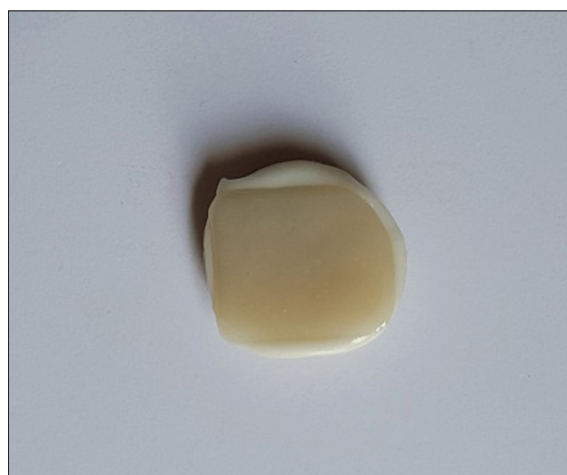
Figure 1: Vita Suprinity sample cemented to composite substrate using white opaque resin cement.
