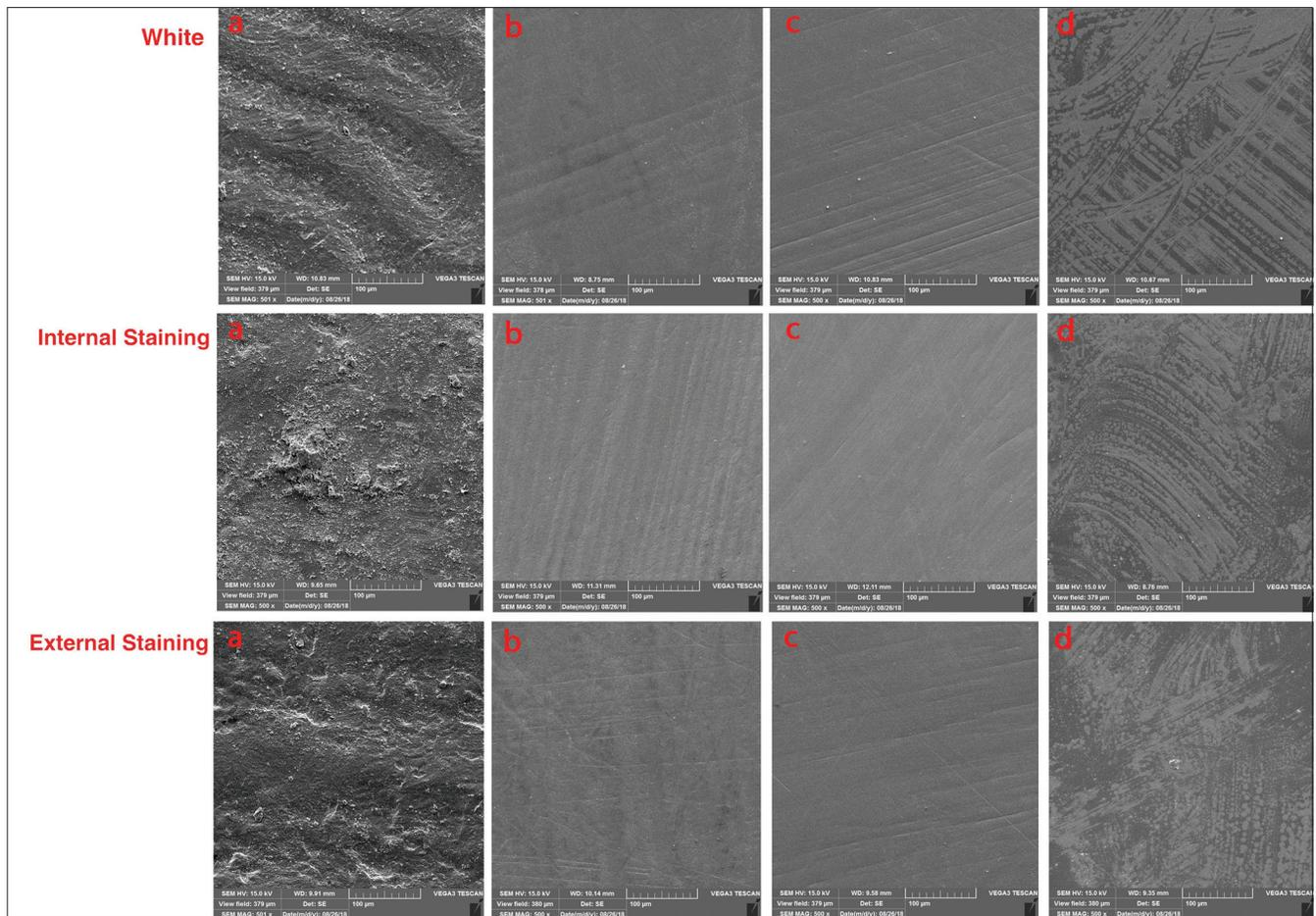
**Figure 6:** Scanning electron micrographs ( $\times 500$ ) of 3 zirconia coloring groups: white, internal staining, external staining. (a) unpolished, (b) polished with Shofu polishing system, (c) polished with dental direct polishing system, (d) glazed.
