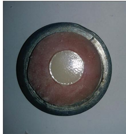
Figure 1: Sample mounted into acrylic resin.
