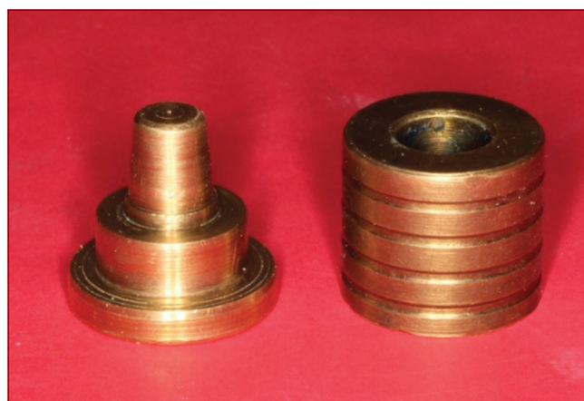
Figure 1: Brass die along with its counterpart.
