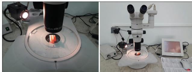
**Figure 1:** Measurement of gap by stereomicroscopy.
