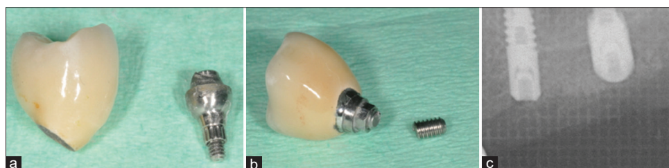
Figure 2: (a) Abutment fractured of the 25 was removed, (b) Abutment screw fractured of the 26 was removed, (c) A radiographic examination excluded radiographical signs of peri-implantitis.
