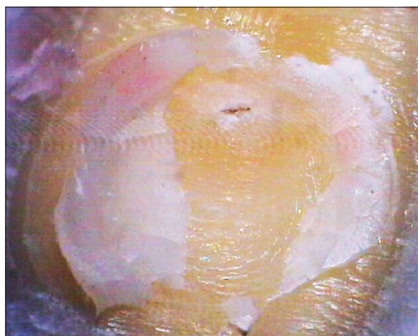
Figure 2: Mix failure of resin-modified glass ionomer sample bonded to dentin bonding surface.
