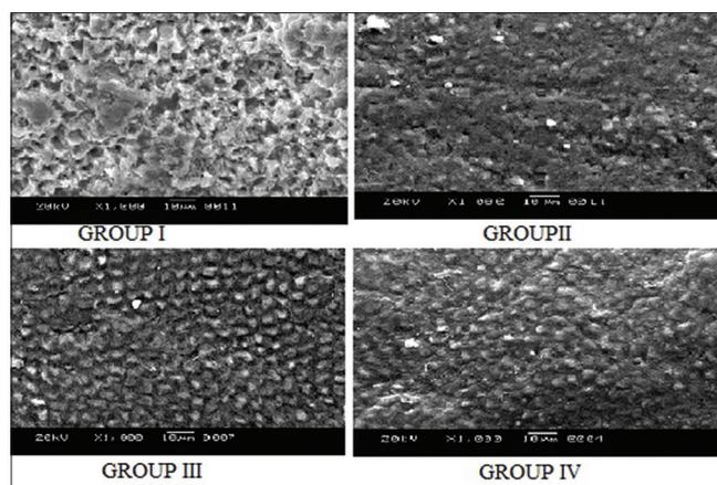
**Figure 2:** Structural analysis of enamel sample by scanning electron microscopy in different group after remineralization.
