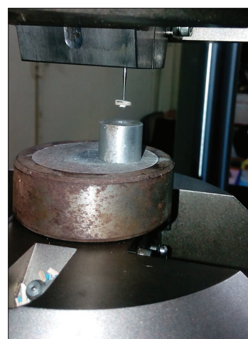
Figure 3: Universal Testing Machine containing cylindrical stainless steel plunger of 1-mm diameter and operating at a speed of 1 \text{ mm/min}^{-1} used to apply force on materials, inside root slices.
