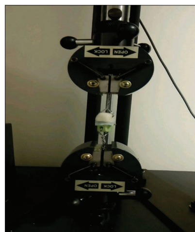
Figure 1: Specimen undergoing bond strength testing in the universal testing machine.
