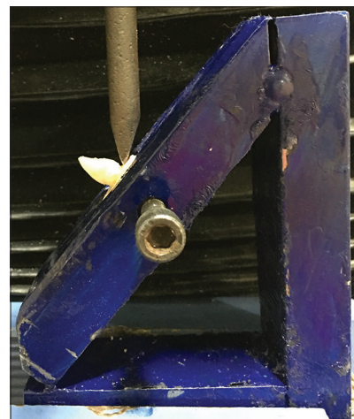
Figure 3: Fracture resistance testing of immature tooth using universal testing machine at an angle of 130°.
