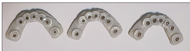
Figure 1: Surgical guide printed by a stereolithography printer.
