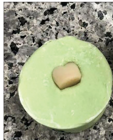
Figure 1: Mounted samples for placement in chewing simulator.
