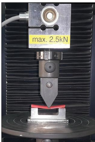
**Figure 2:** Three-point bending setup for fracture test.
