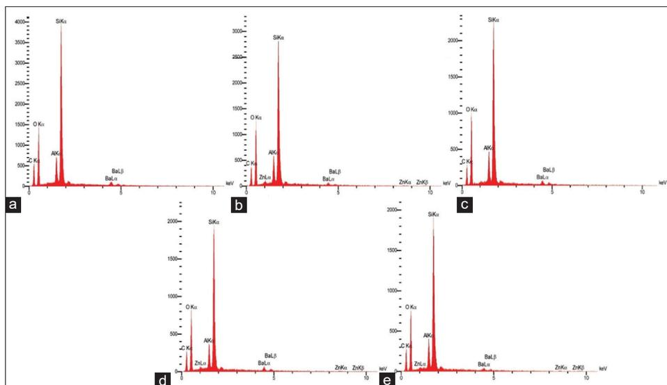
**Figure 4:** X-ray diffraction charts of composite discs. (a) Without powder, (b) With zinc oxide powder, (c) With graphene oxide, (d) With physical compound of graphene oxide and zinc oxide, (e) With chemical compound of graphene oxide and zinc oxide.
