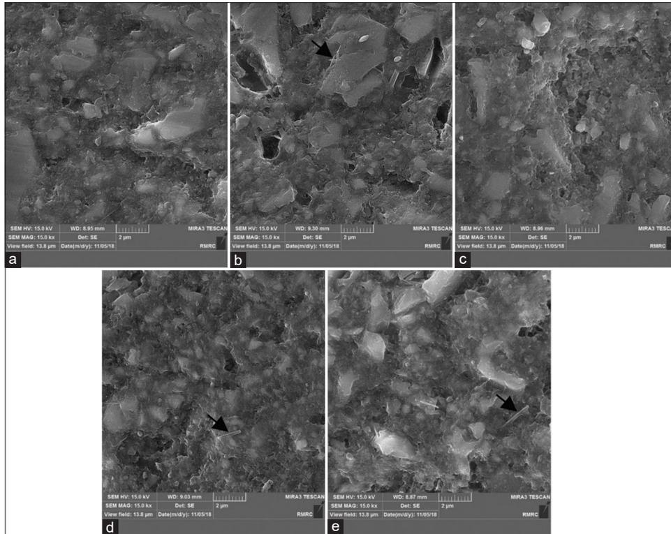
**Figure 2:** Scanning electron microscopy images of composite discs ( $\times 15K$ ). (a) Without powder, (b) With zinc oxide powder, (c) With graphene oxide powder, (d) With physical compound of graphene oxide and zinc oxide, (e) With chemical compound of graphene oxide and zinc oxide.
