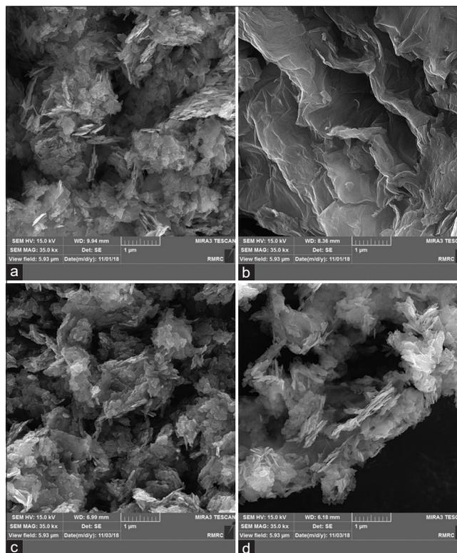
**Figure 1:** Scanning electron microscopy images of nanoparticle powders ( $\times 35K$ ). (a) Zinc oxide powder, (b) Graphene oxide powder, (c) Physical compound of graphene oxide and zinc oxide, (d) Chemical compound of graphene oxide and zinc oxide.
