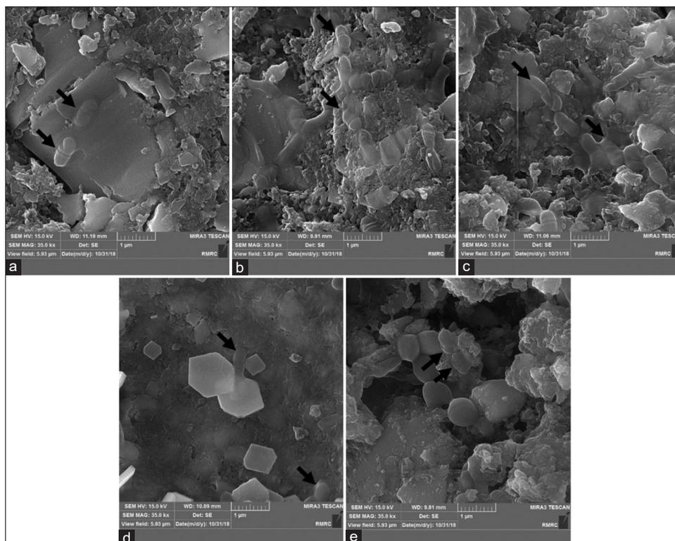
**Figure 5:** Scanning electron microscopy images of microbial adherence to composite discs ( $\times 35K$ ). (a) Without powder, (b) With Zinc oxide powder, (c) With graphene oxide, (d) With physical compound of graphene oxide and Zinc oxide, (e) With chemical compound of graphene oxide and zinc oxide.
