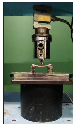
Figure 16: Plastic deformation under load in the 3-point bend test.
