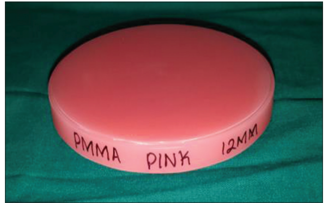
Figure 7: PMMA IvoBase® CAD Resin Block. PMMA: Polymethyl methacrylate.
