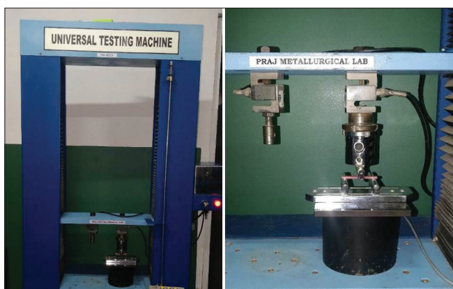
Figure 15: Specimens being 3-point bending tested in Universal Testing Machine.
