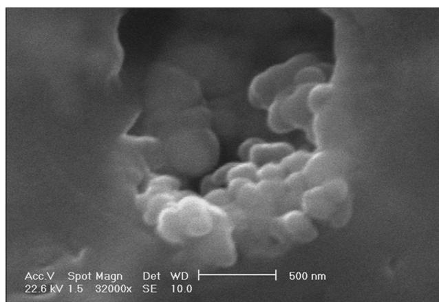
**Figure 2:** The SEM image showing an average particle size of 17.145 nm in the agglomerate state. SEM: Scanning electron microscopy.
