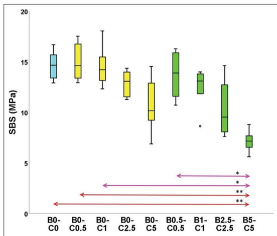
**Figure 5:** Box plots showing descriptive SBS statistics (MPa). Significant Dunn pairwise comparisons are marked with double-arrows: \* $P < 0.05$ ; \*\* $P < 0.01$ . SBS: Shear bond strength; MPa: Mega Pascal.
