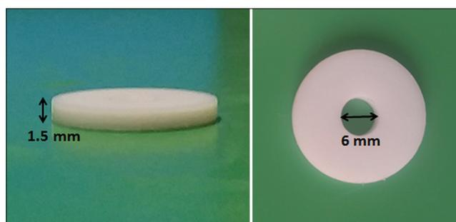
**Figure 3:** The custom-made cylindrical polytetrafluoroethylene mold.
