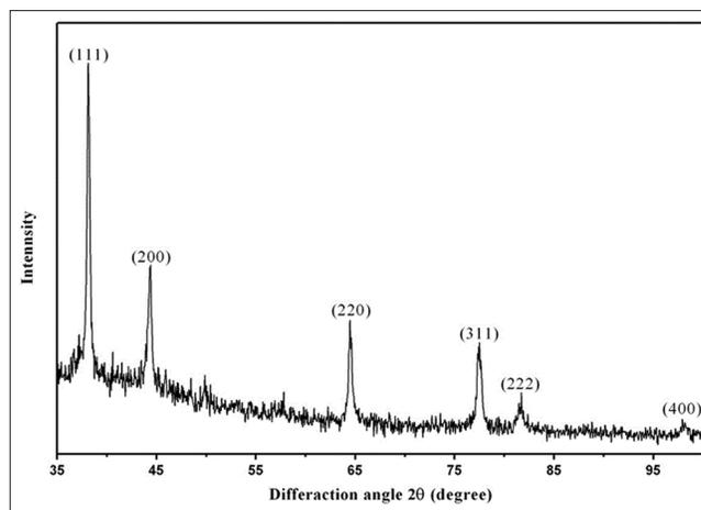
**Figure 1:** The XRD pattern showing silver particles of high purity. XRD: X-ray diffraction.
