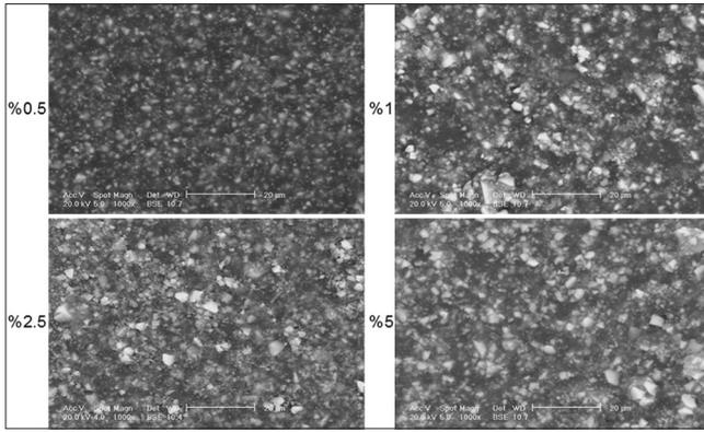
**Figure 4:** Composite discs at × 1000 confirming relatively uniform distribution of nanosilver.
