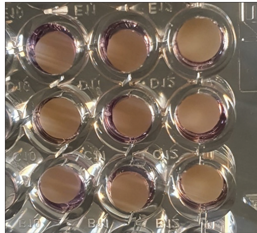
Figure 3: Direct 3-(4,5-dimethylthiazol-2-yl)-2,5-diphenyltetrazolium bromide cell assay. The samples are simple, glazed, and polished from left to right.
