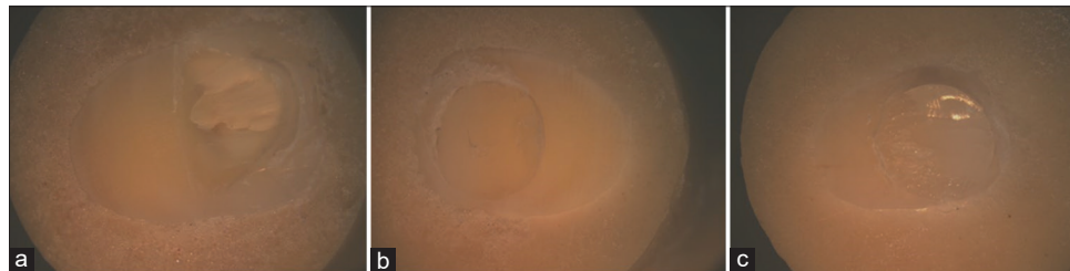
Figure 2: (a) Showing cohesive failure within the tooth itself. (b) Adhesive failure. (c) Mixed failure for Group I specimens.
