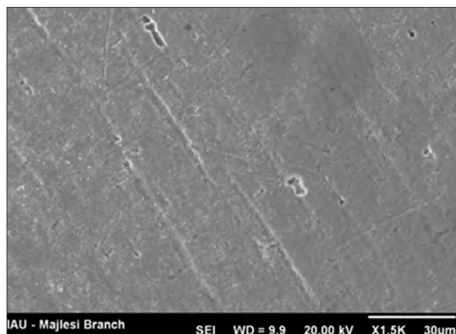
Figure 5: 0.019 × 0.025 inch NiTi in Aquafresh solution
