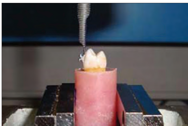
Figure 5: Placing the blade of Zwick machine vertically between the base of the bracket and the resin (lateral view)
