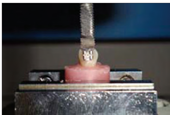
Figure 6: Placing the blade of Zwick machine vertically between the base of the bracket and the resin (frontal view)
