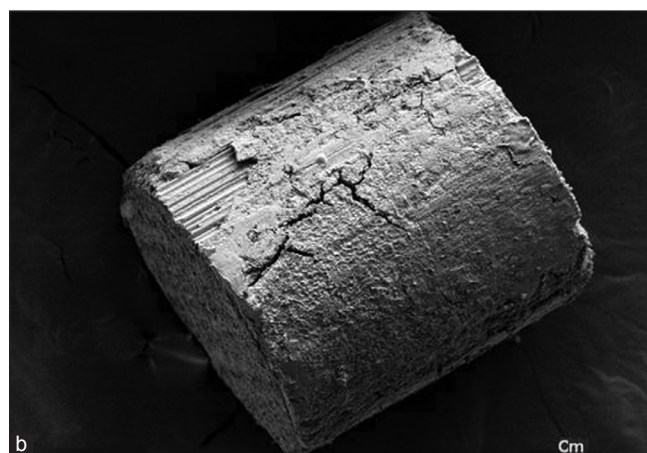
Figure1: Scanning electron microscopy images from push-out tested specimens. Cohesive failure in post in G3 (a) and G4 (b)
